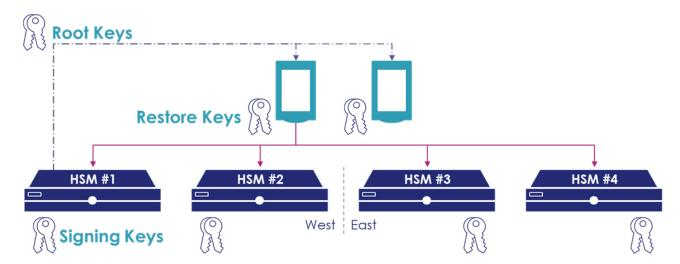
This architecture can tolerate the loss of all production Network HSMs and all but one USB-based HSM. It also allows for the introduction new Thales HSMs later in the products' lifecycles. Upon hardware failure or decommissioning, new Network HSMs can be brought online, one of the USB-based HSMs brought out of storage, and the spare OTS private keys on a Restore Key used to sign newly generated Signing Keys.
