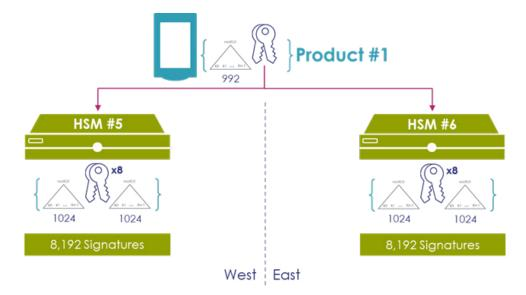
In this configuration, the signature scheme can tolerate the loss of all production Network HSMs as well as accept the introduction of new Thales HSMs later in the products' lifecycles. Upon hardware failure or decommissioning, new Network HSMs can be brought online, the USBbased HSM brought out of storage, and the spare OTS private keys on the Root Key used to sign newly generated Signing Keys.
