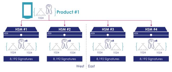
Here, the Root Key is generated with a set of 1,024 OTS private keys, while the same Signing Keys are generated on the Network HSMs. Then, the Tablet HSM can be taken offline and put into cold storage.
